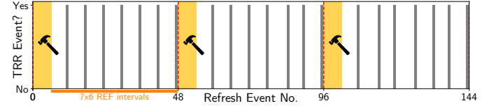
Fig. 16: Attack strategy. The refresh interval range 0 – 144 of Figure 15 zoomed-in. We show the distance between TRR-free segments (every 48-th interval, red lines), the 6 refresh intervals where we target hammering our aggressors (yellow), and the 7 \times 6 intervals where we hammer two random rows (orange).
