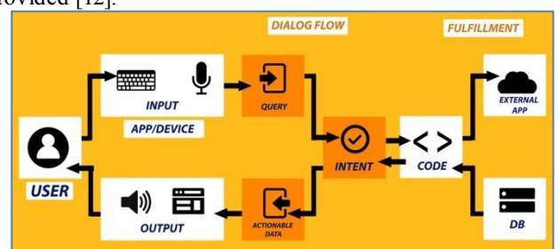
Fig 1. The Architecture of the Conversational Bot
