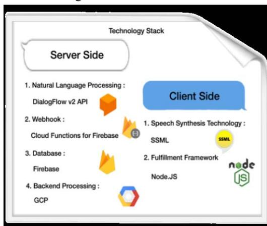
Fig 2. Technology Stack used for "Aapka Chikitsak"
