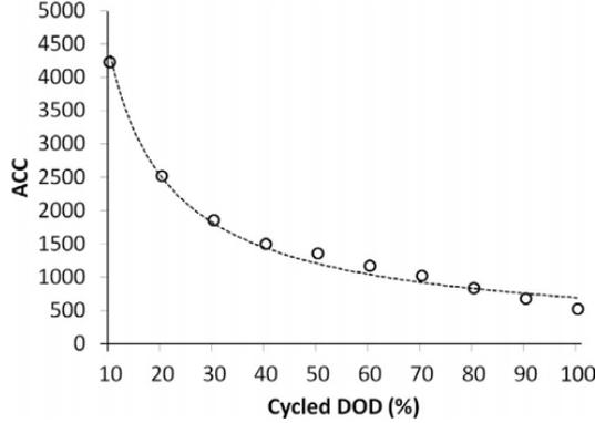
Figure 1. A lithium-ion DOD-ACC cycle life Model [6]
