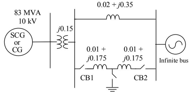
Figure 1. Configuration of the simulated single-machine infinite bus system.
