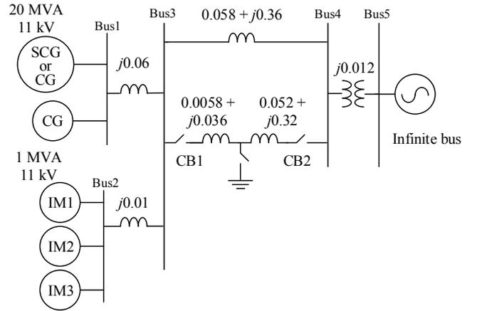
Figure 3. Configuration of the simulated double-machine infinite bus system
