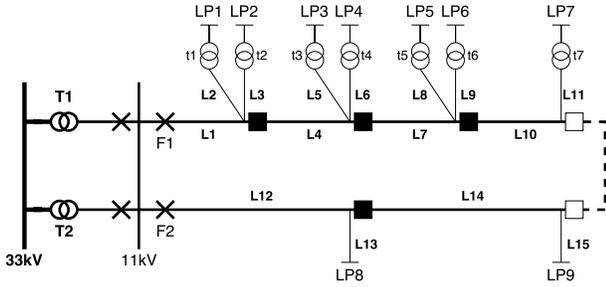
Fig. 1: Feeder 1 and 2 of the RBTS Bus 2 distribution grid test system, adapted from [8].
