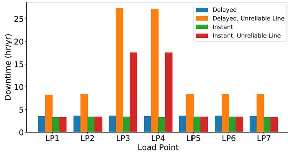
Fig. 5: Downtime of each load point before and after setting L4 MTTF to 1% of its value, with delayed and instant reconfiguration.
