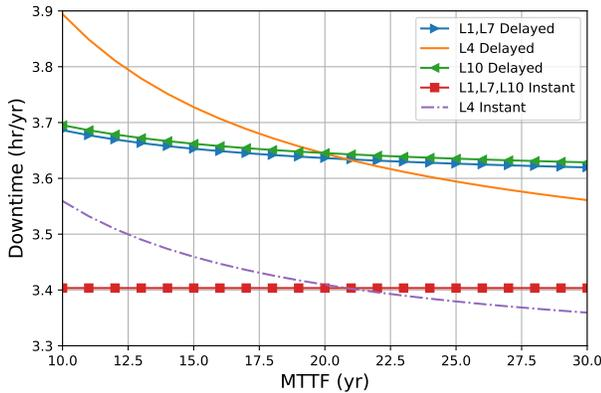
Fig. 3: Downtime of LP1 for varied feeder line MTTF, for delayed and instantaneous reconfiguration
