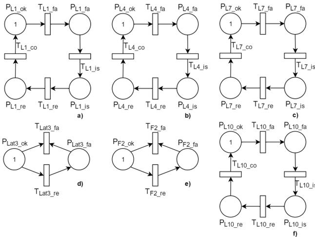
Fig. 2: SRN used to model availability of LP3 on Feeder 1
