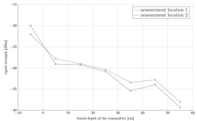
Fig. 4. Received signal strength for various depths
