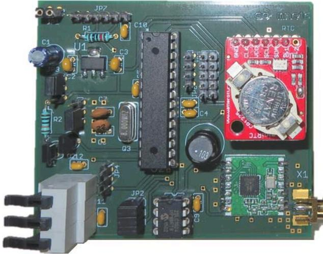
Fig. 2. Top view of the MoleNet sensor node
