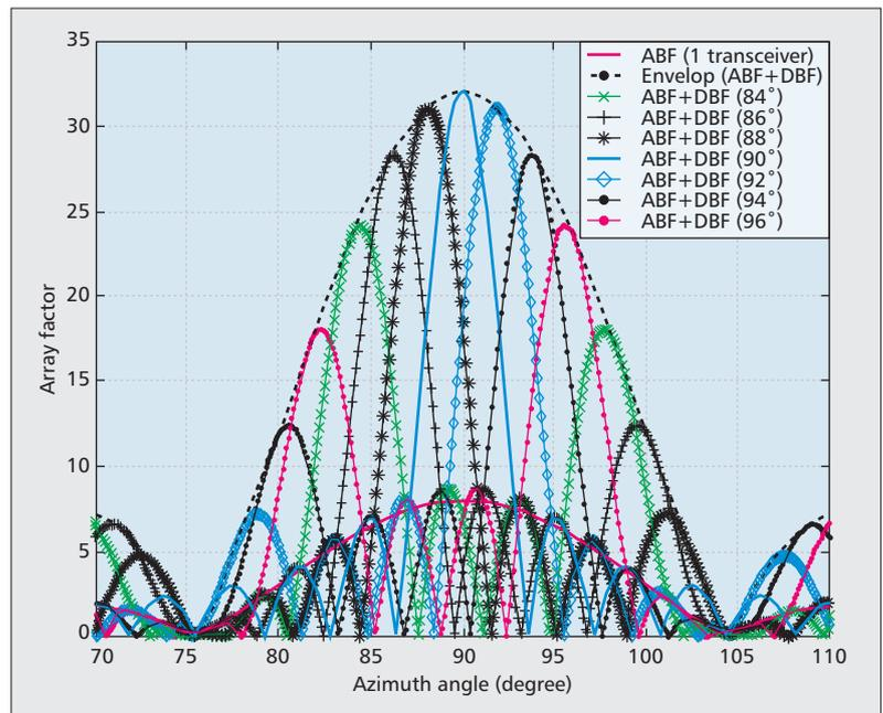
Figure 6. Hybrid BF with a 32-element antenna array.
