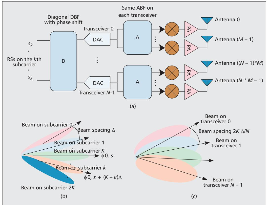
**Figure 5.** RS design for the  $N \times M$  hybrid BF structure: a) hybrid BF for beam domain RSs; b) beam domain RSs with hybrid BF on different subcarriers; c) beam domain RSs with  $M$  antenna analog BF.
