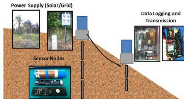
Figure 2. System diagram of the landslide monitoring system consisting of the sensor columns, data logging and transmission unit, and the power source which can be from the grid or solar.
