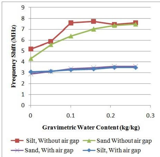
Figure 9. The results of the characterization of the soil moisture sensor with air gap and without air gap in both sand and silt showing improvement in the sensitivity and dynamic range of the soil moisture sensor after removing the air gap.
