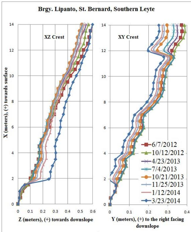
Figure 5. Initial significant tilt data obtained from the sensor column installed in the crest part of the slope in Benguet and Southern Leyte sites.
