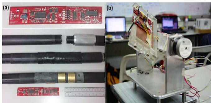
Figure 6. (a) The redesigned sensor board and packaging prototype showing the mechanical segment coupler, segment enclosure with heat shrinkable tube outer layer, the exposed soil moisture capacitor electrodes (brass) and the sensor board with dual accelerometer and soil moisture board. The diameter of the pipe segment was reduced in the new design for easier transportation and insertion in the borehole. (b) The 3 DOF calibration gimbal with sensor boards attached for calibrating accelerometers.
