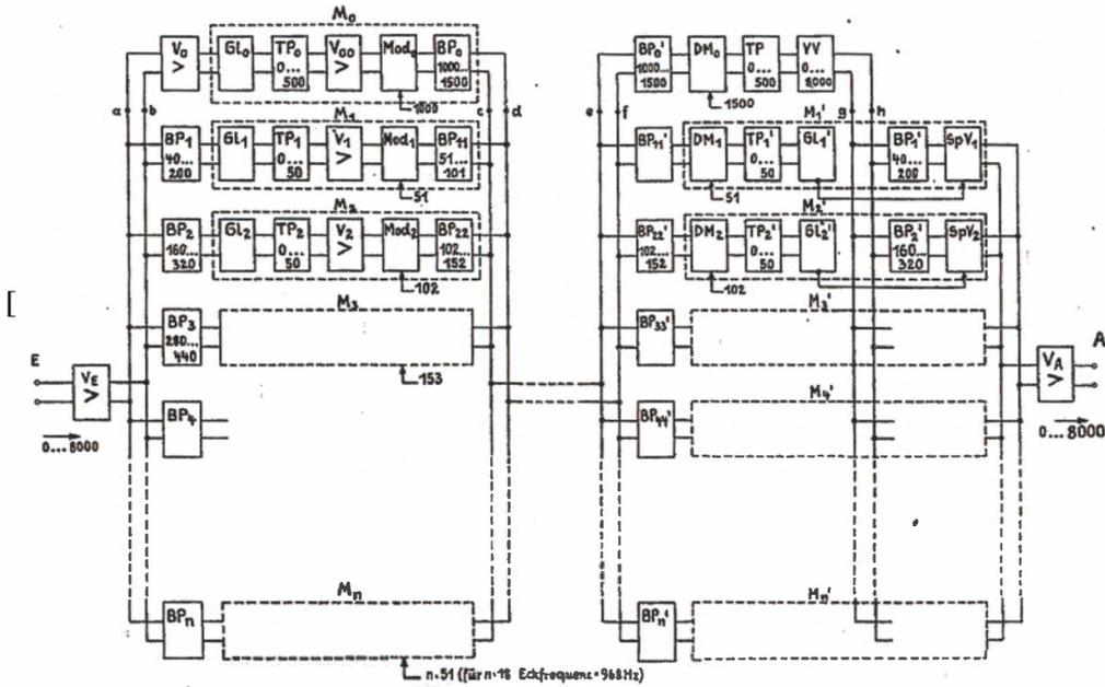
Fig. 3. Block diagram of the transmission system of K. O. Schmidt according to the patent [19]. The part below the line a-h represents the frequency channels according to the basic patent from 1932 [18]. The part above this line extracts and adds the information on voiced / unvoiced signal segments and (in the case of voiced signals) the fundamental frequency. This part forms the content of the supplementary patent from 1939 [19].
