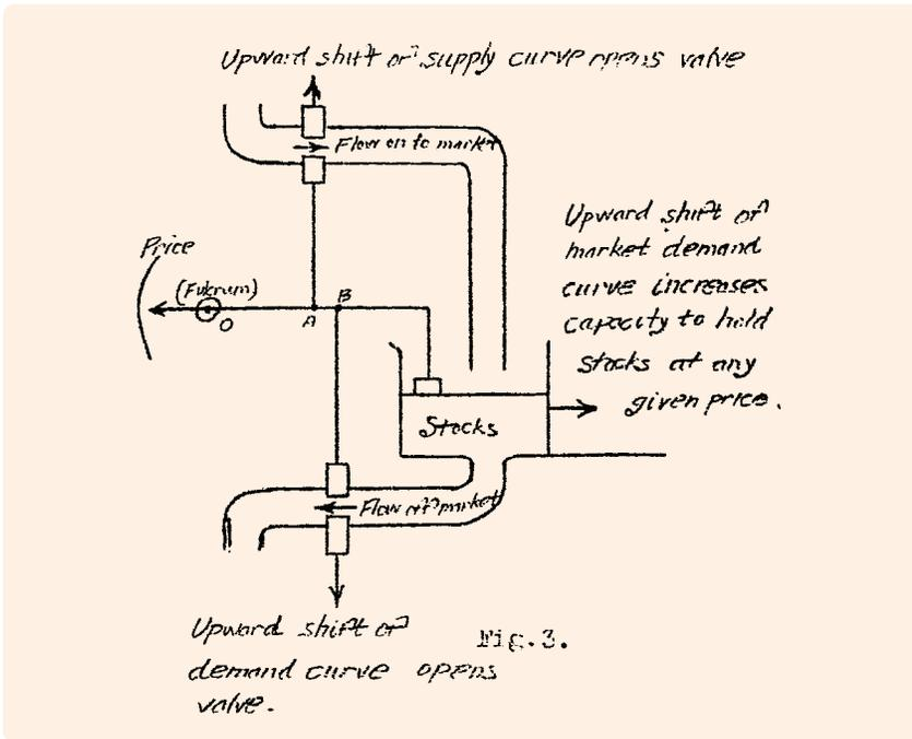
**FIGURE 3** Phillips's sketch of the fundamental component of a hydraulic simulator of an economy, from an unpublished paper now in the possession of Martin Slater, Fellow of St. Edmund Hall, Oxford. This paper was the stimulus for building the prototype machine.
