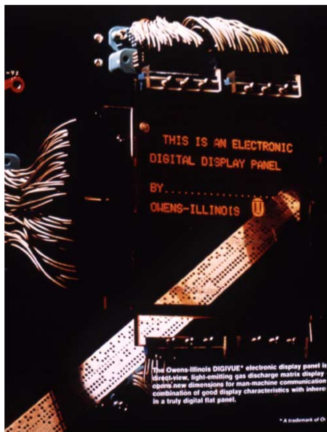
Fig. 7. Open-cell structure was used in this 128 \times 128 pixel plasma display developed by Owens Illinois in 1968 which measured 4 in \times 4 in. This was the first practical and manufacturable structure. It used a robust 6-mm-thick glass substrate, thick film gold electrodes, and a screen printed solder glass dielectric layer. A very similar structure is used for all of today's plasma TV front plates. This display was transparent as demonstrated by the punch tape in the background.
