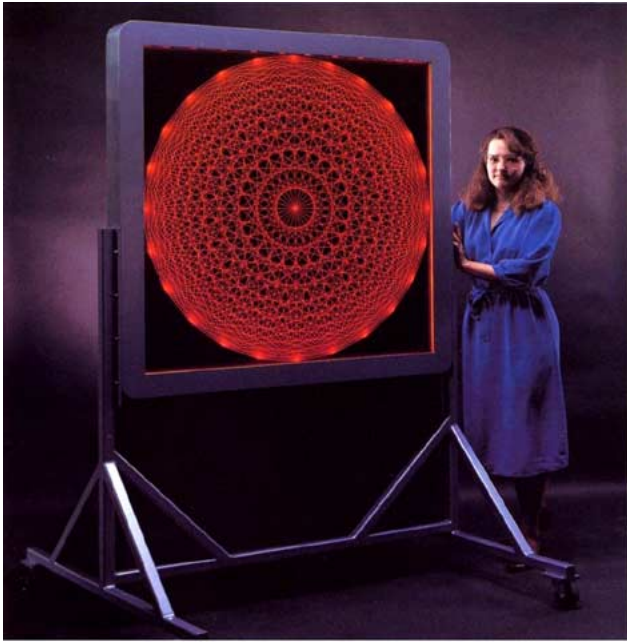
Fig. 17. The 59-in diagonal product with 2048 \times 2048 monochrome pixels developed by Photonics in 1987 [29]. This product clearly demonstrated that large size plasma displays were possible. This presented good proof that the issues of electrode resistance, inductance, panel capacitance, and addressability of such large panels were manageable.
