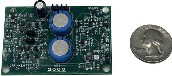
Fig. 8. Photograph of the top side of the energy management PCB prototype with a United States quarter coin for scale reference.
