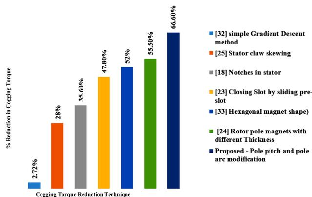
**FIGURE 27.** Comparison of cogging torque reduction techniques.
