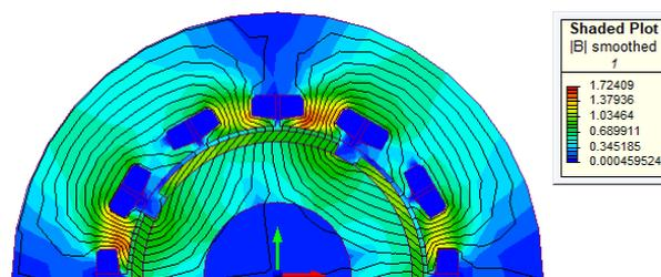
**FIGURE 2. Flux density distribution in symmetrical structure.**
