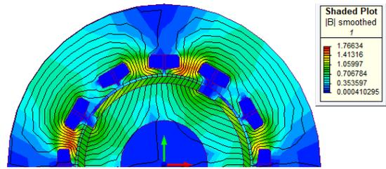
FIGURE 21. Flux plots in proposed BLDC motor.
