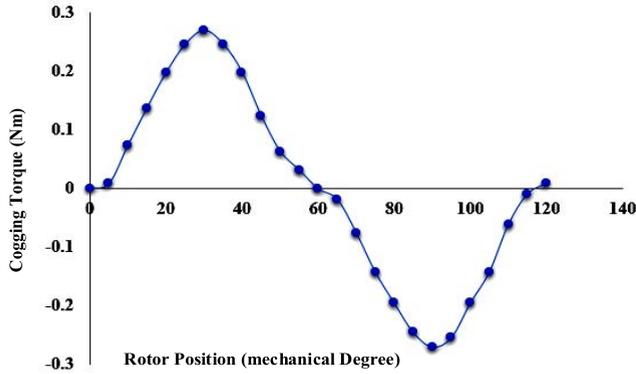
FIGURE 3. Cogging torque of conventional BLDC motor.
