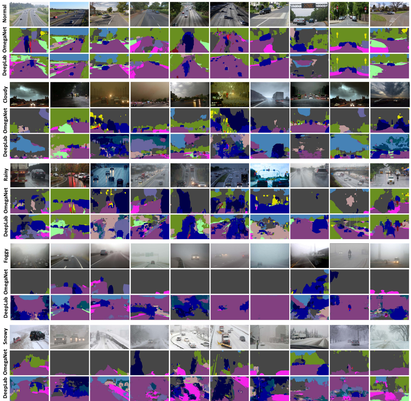
Fig. 5. Visual segmentation results of various deep segmentation models over input images having variable weather conditions such as snow and fog. The segmented maps of DeepLab and OmegaNet are not trustworthy for an autonomous vehicle’s scene understanding.
