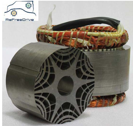
Fig. 13. Wound stator core and rotor core of the CCV SynRel.
