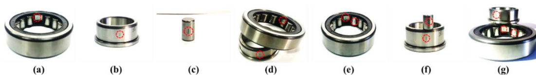
FIGURE 9. Rolling bearing fault types: (a) outer race defect (ORD), (b) inner race defect (IRD), (c) roller defect (RD), (d) inner and outer race defect (IORD), (e) outer race and roller defect (ORRD), (f) inner race and roller (IRRD), (g) inner race, outer race, and roller (IORRD).
