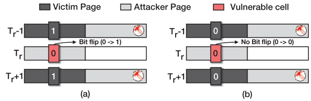
Fig. 1: Data dependency for inducing a rowhammer fault. Here, based on the presence of bit flip in the attacker-controlled vulnerable bit in the target row ( T_r ), data from adjacent row from victim program can be inferred.
