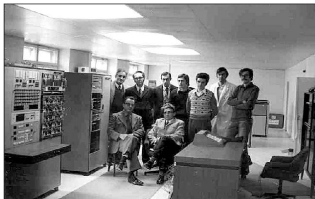
Fig. 4 The photo shows an analog part of the HRS-100 computer, a box with A / D and D / A converters, a table with a control console and part of the development team. Source: [40]
