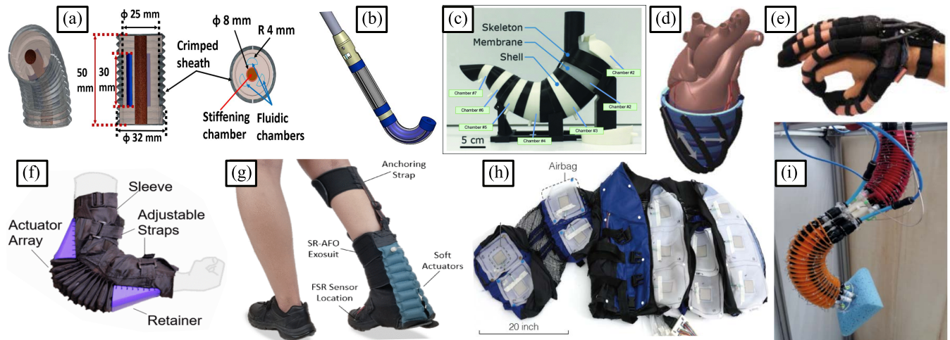
FIGURE 9. Biomedical application of pneumatic soft robotics: (a) STIFF-FLOP [566], (b) novel STIFF-FLOP with fiber jamming [368], (c) soft robotic gastric simulator [567], (d) soft robotic heart sleeve [568], (e) soft robotic glove [569], (f) soft elbow exosuit [570], (g) soft robotic ankle-foot orthosis exosuit [571], (h) pneumatic force jacket [572], and (i) I-support soft arm for bathing assistance [564]. All figures are reproduced with permission.
