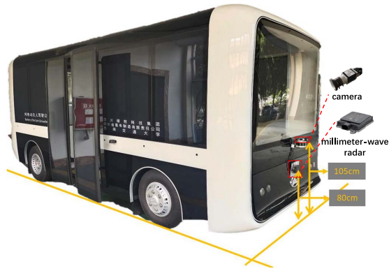
Fig. 7. Millimeter-wave radar and camera installation position diagram.
