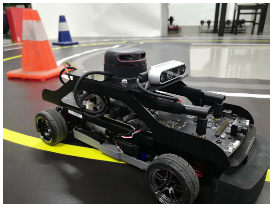
Fig. 11. QCar: a small-size autonomous vehicle platform.
