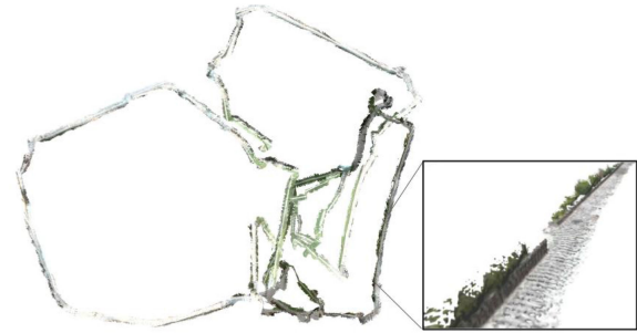
Fig. 15. Stata experiment . Optimized mesh produced by Kimera-Multi corresponding to trajectory estimate shown in Fig. 14(c).
