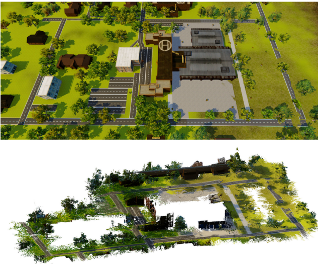
Fig. 13. Dense metric 3-D mesh model generated by Kimera-Multi with three robots in the simulated Medfield scene.
