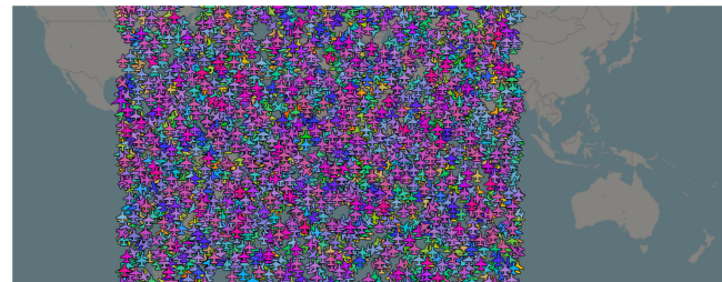
Fig. 6. Flooded screen when using tar1090 software.
