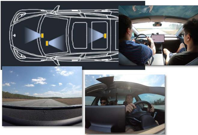
Fig. 4. Video camera setup. Road camera on left, console camera on upper right and driver camera on lower right.
