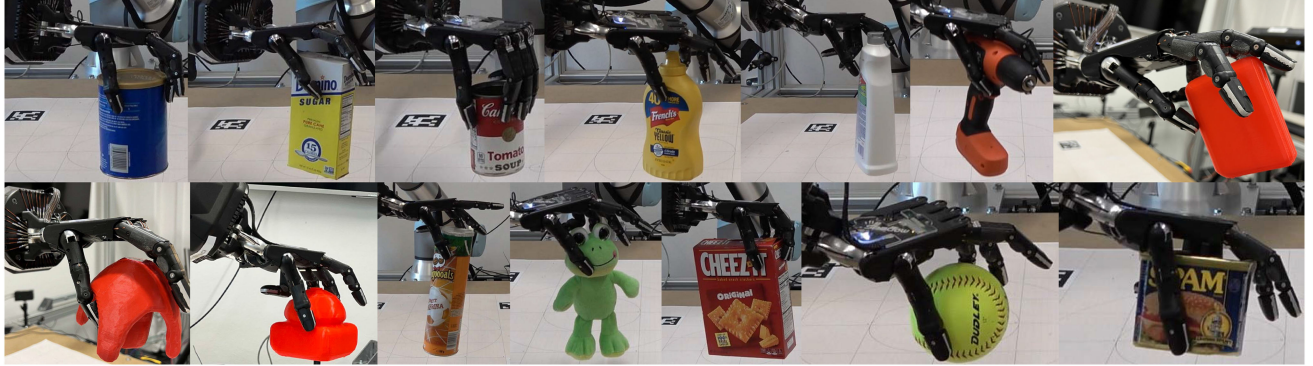
Fig. 8. Grasp examples for each object. The agent used in these grasps is GRU-M3PCA5.
