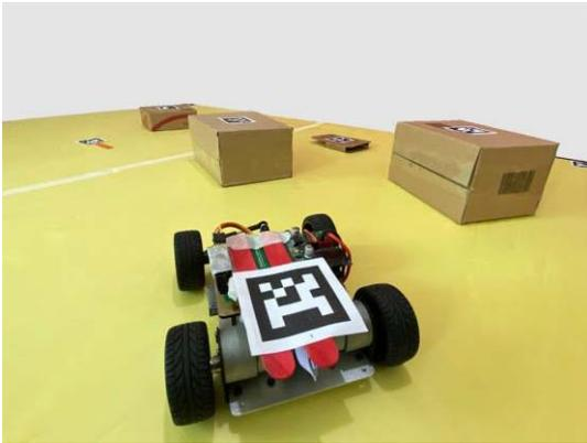
Fig. 9. Experimental platform based on an ackermann-steering car-like robot.
