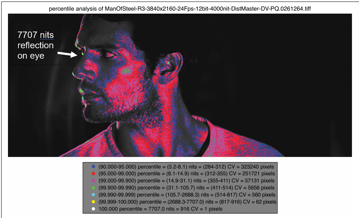
FIGURE 6. Example frame containing the single brightest pixel of the film overlaid with a percentile heat map.
