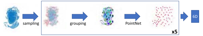
Fig. 15. Diagram of the algorithm proposed by Hu et al. [51] to estimate head pose of the driver using point cloud data. The framework directly uses the point cloud data without projecting the 3D points into 2D spaces.
