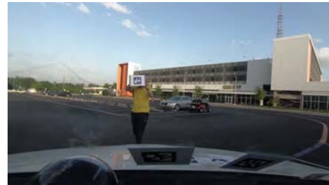
Fig. 2. Step 1 in the data collection protocol. The driver looks at a target board with a fiducial mark held by one of the researchers outside the car. This part in the protocol provides continuous gaze information.
