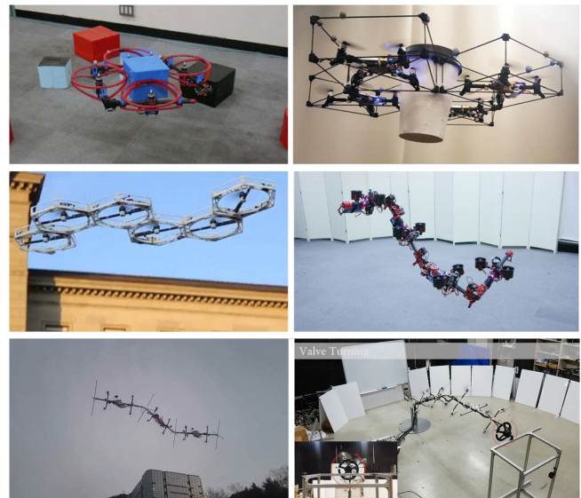
Fig. 5. Examples of interconnected actuated multibody designs (from top, from left): 1) HYDRUS [105]; 2) flying-gripper [146]; 3) DFA [147]; 4) DRAGON [148]; 5) flying LASDRA [149]; and 6) operation LASDRA [109].
