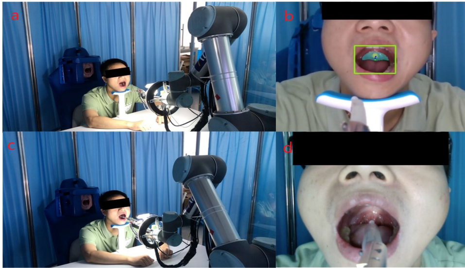
Fig. 9. Sampling process from vision detection to sampling tasks. In our experiments, many volunteers were tested, and the recognition rate, control precision, sampling time, and sampling contact force were recorded.
