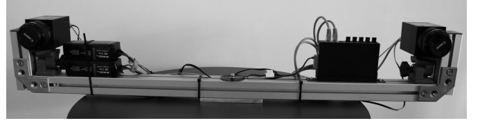
Fig. 4. Our stereo camera pair setup. Two cameras, ethernet switch, and two batteries mounted on an aluminium profile.
