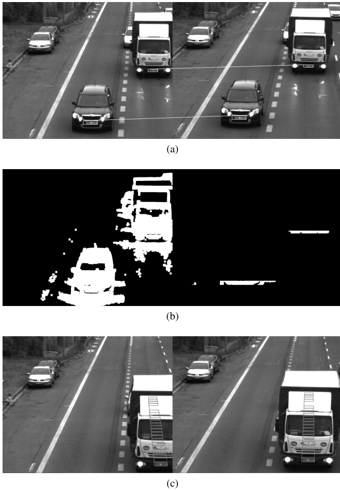
Fig. 2. License plates detection and tracking. (a) Detected license plates in the image from the camera on the left and their matching counterparts in the right camera image forming a license plate pairs. (b) The license plates search areas in both images were constrained by foreground masks constructed using background subtraction. The right image search area was further constrained using epipolar geometry. (c) A vehicle with its set of all license plate pairs.
