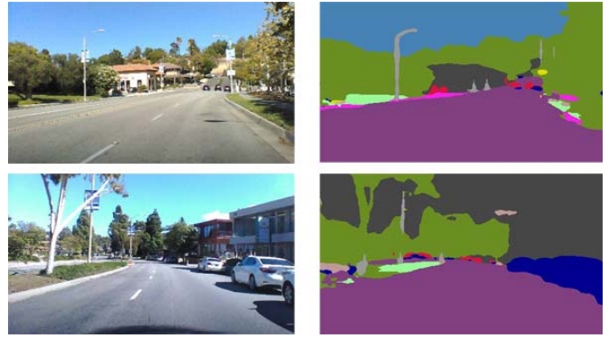
Fig. 5. Real images from the driving data and their semantic segmentations (source: [72]).
