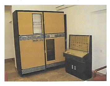
In 1967 begun the design of GOLEM B, with 64-bit words, but with a memory of 128K words. It was a fast machine, using emitter-coupled logic and multi-layer circuits. This computer became operational in 1974 and was active until 1983.
