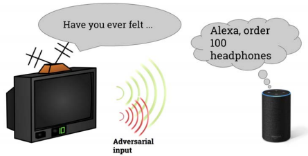
Fig. 1. Example of targeted adversarial attack on speech to text systems in practice
