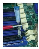
(b) Tweezers short-circuiting  $DQ_0$  and  $V_{SS}$ . (a) A custom shunt probe.
