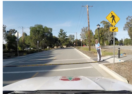
Fig. 2. Experimental setup of pedestrian crosswalk using a cardboard cutout for the pedestrian that moves along a track. Depicts the pedestrian posture of stopped.
