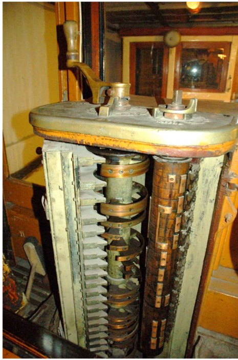
Fig. 6.: „BSzKRt” type controller from the thirties in the carriage No.19 in the URM
