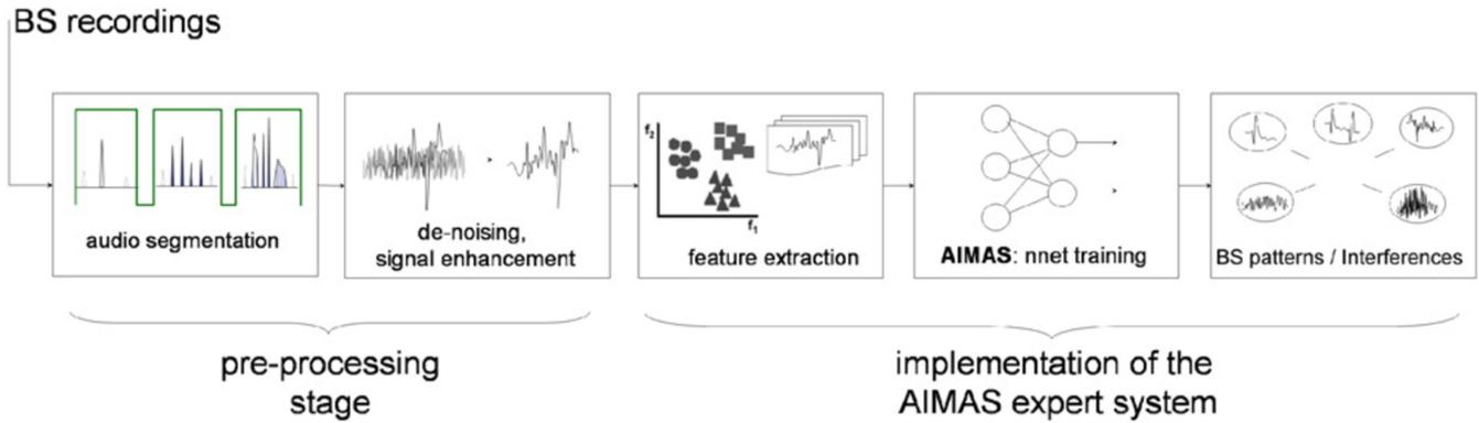
Fig. 8. Development phases of the AIMAS project, [12].
