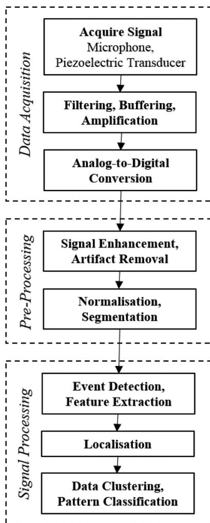
Fig. 3. Bowel sound signal processing flow chart.
