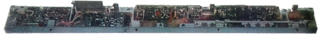
Fig. 1. Selectric Bug, one of the first keylogging side channel attacks discovered in the wild. Reprinted with permission from [4] and on display in the National Cryptologic Museum.
