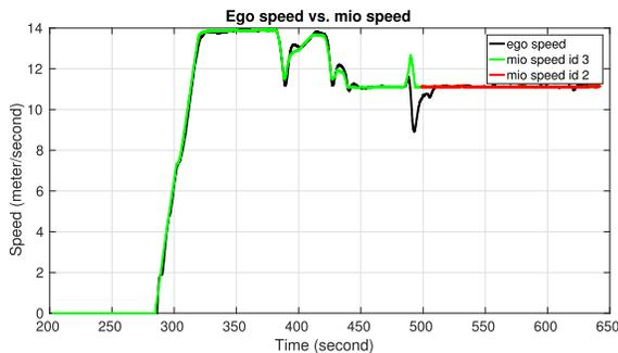
Fig. 10. CACC vehicle speeds during the merging heat.
