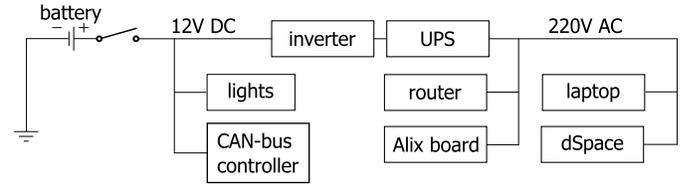
Fig. 2. Power supply setup for the system.
