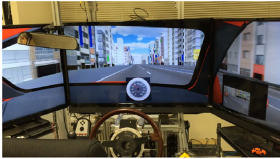
Fig. 1. Driving simulator and course.
