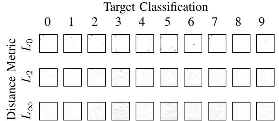
Fig. 7. Targeted attacks for each of the 10 MNIST digits where the starting image is totally white for each of the three distance metrics.
