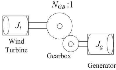
Fig. 3. Two-mass model of drive train.
