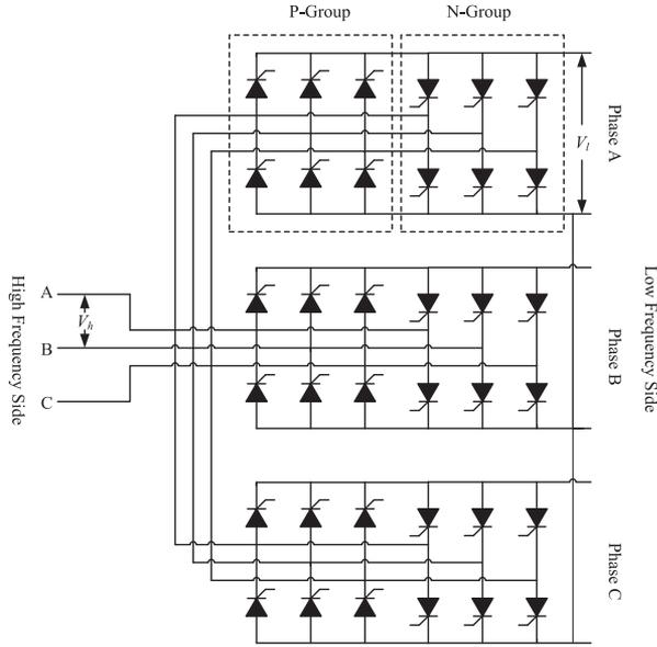
Fig. 6. Structure of a three phase cycloconverter.
