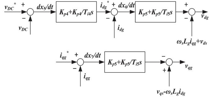
Fig. 5. Control block diagram of grid-side converter.
