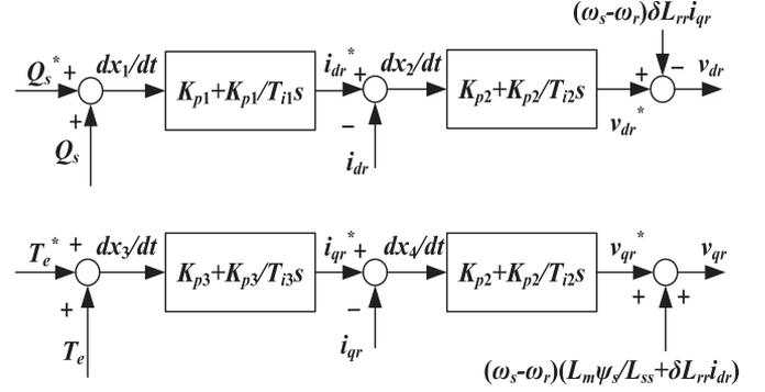
Fig. 4. Control block diagram of rotor-side converter.
