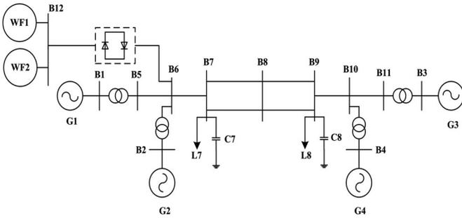
Fig. 10. Configuration of the simulations in four-machine system.
