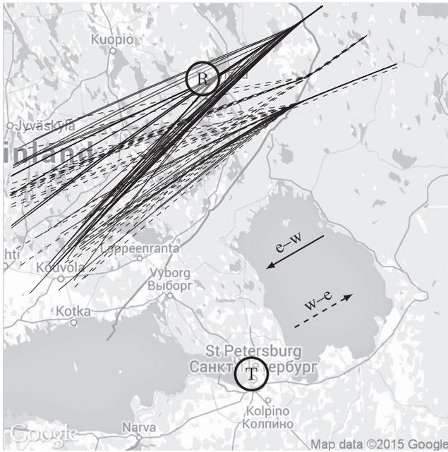
Fig. 1. Geographical location of transmitter T, receiver R, and trajectories of FR24 data. Solid and dashed lines correspond to e-w and w-e azimuths, respectively.
