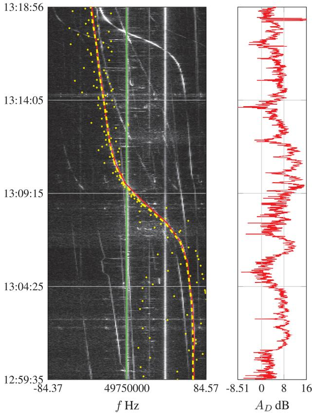
Fig. 4. Spectrogram: yellow dots—Doppler shift based on FR24 data  $f_D^{\text{FR24}}$ ; yellow dashed line—smoothed Doppler shift based on FR24 data  $f_D^{\text{FR24*}}$ ; red line—extracted Doppler curve  $f_D^{\text{RSD}}$ ; green line—extracted carrier  $f_c$ . Right: amplitude of extracted Doppler signature  $A_D$ .
