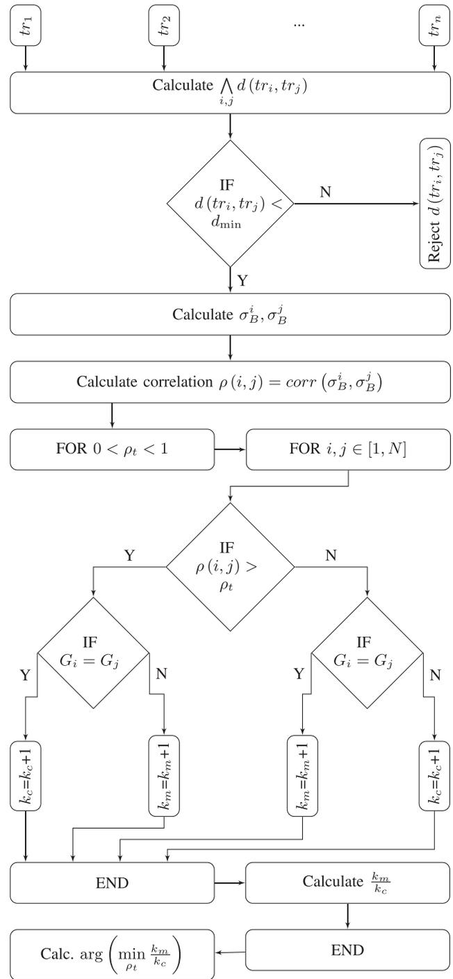
Fig. 8. Procedure of estimating optimal correlation threshold whose effects are presented in Fig. 7.
