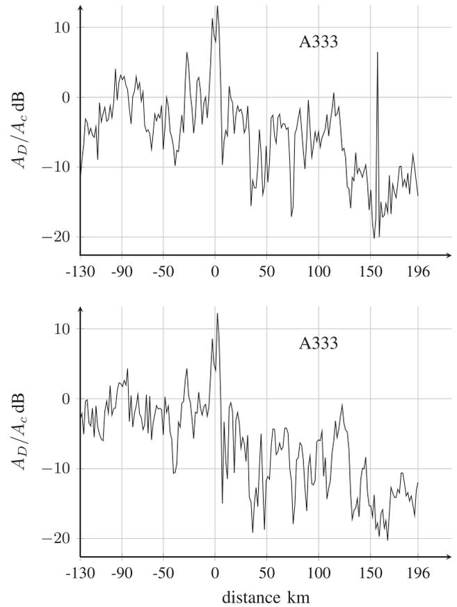
Fig. 6. Fraction of reflected to direct signal from two Airbus A330-300 aircrafts in time domain.
