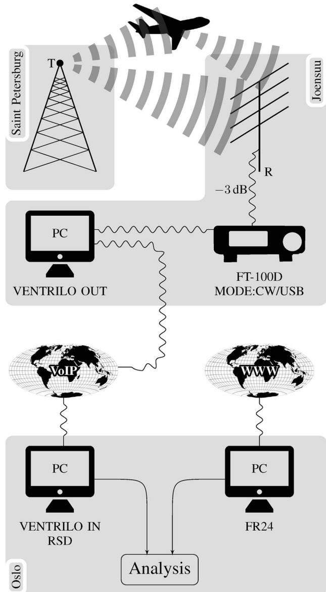
Fig. 2. Equipment (sources) used for collecting RSD and FR24.
