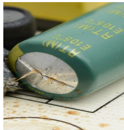
Fig. 3. Failed electrolytic capacitor from an LED luminaire driver circuit. Failure resulted in venting of the electrolyte as shown by the brown electrolyte residue on the printed circuit board and the breach in the vent on the top of the capacitor.
