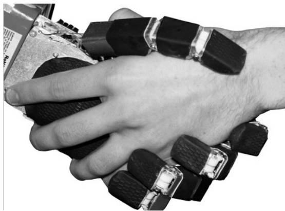
Fig. 3. The Dextrus hand is a 3D printed, myoelectric prosthesis for amputees with above the wrist amputation.
