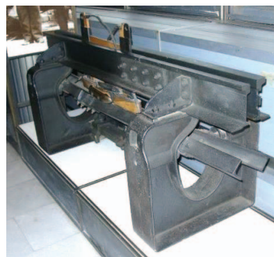
Fig. 2.: The lower current collector system in the Budapest Transportation Museum (Varga Ákos Endre – [8])
