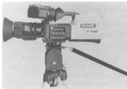
Figure J-13. Single tube color camera (NHK).
