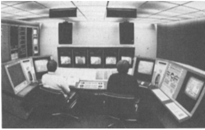
Figure UK-18. First of a new generation of Regional Operations Centers opened at Emley Moor. More than 550 unattended transmitters are now controlled from four ROCs.
