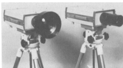
Figure J-21. Optical communication equipment for relaying TV signal (R. transmitter; L. receiver).
