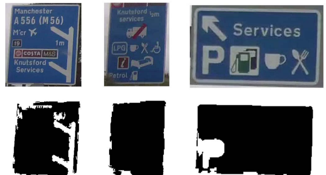
Fig. 11. Example noisy traffic sign candidates shown with their corresponding HSV threshold CCs.
