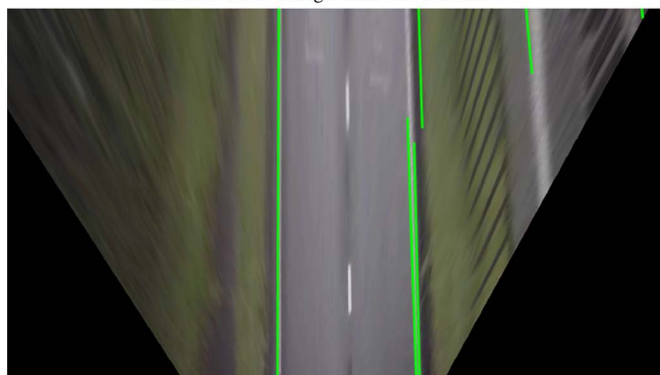
Image and Hough lines with inverse perspective transform performed
