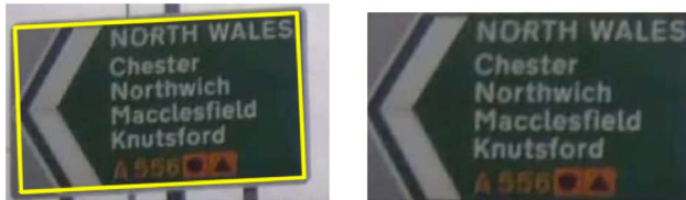
Correction of non-quadrilateral detected region, showing detected quadrilateral (left) and corrected region (right)
