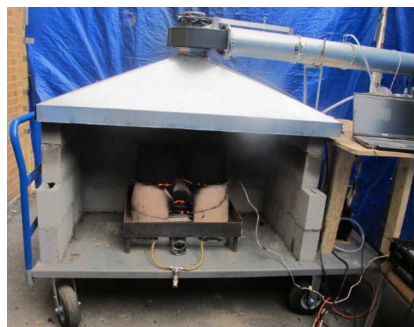
Fig. 2. Picture of the Replica of a Traditional Peruvian Cookstove Used in the Biomass Cookstove Test Facility
